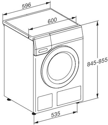
WT1 8/5 kg, drawing, slanted facia, straight facia, mesures in mm
