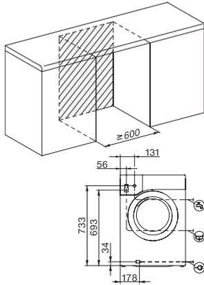
WT1 8/5 kg, installation drawing, slanted facia, straight facia, mesures in mm
